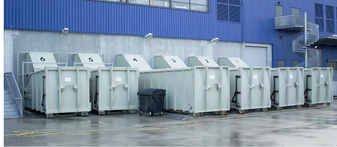
Transport containers at static compactor facility
