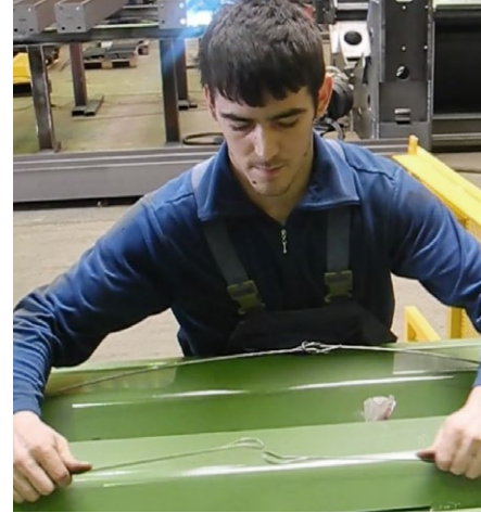
Manual binding with prefabricated quick-tie wires
