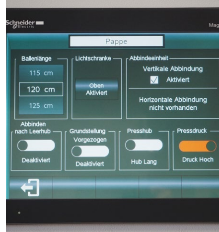
Touchscreen display with individual settings for pressing different materials
