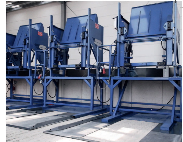
Ramp installation of static bin-lift devices
