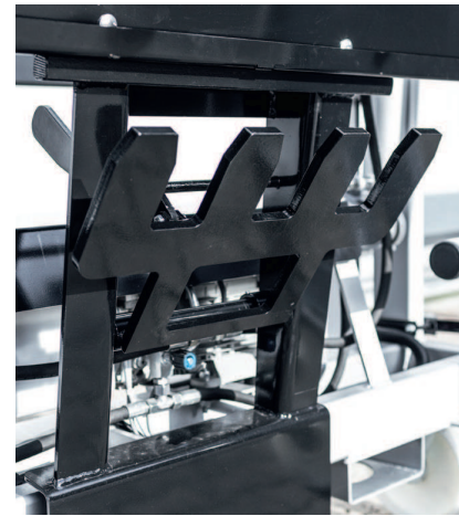
Mechanical lifting comb for 120/240 l containers
