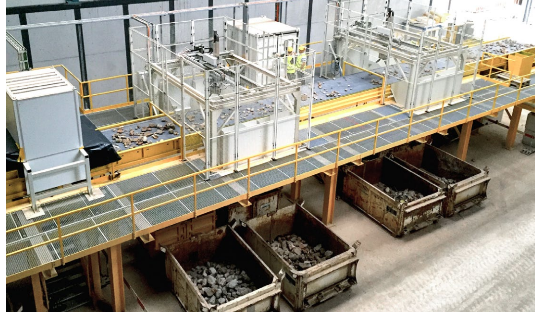
Sorting belt for fully automated robot sorting
