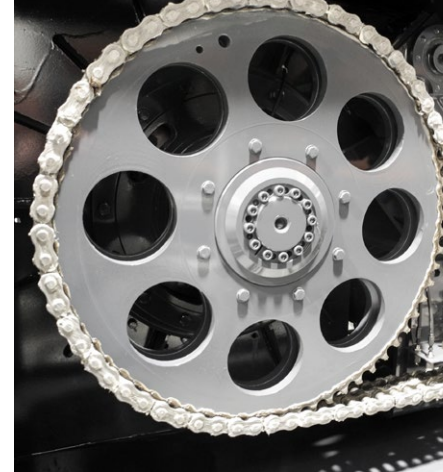
Duplex chain drive (15kW)
