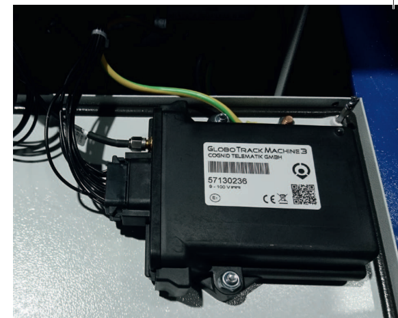
GTM installation on the cover of the switch box and connection to the Avermann circuit board
