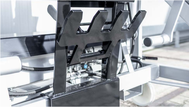
Mechanical lifting comb for 120/240 l containers
