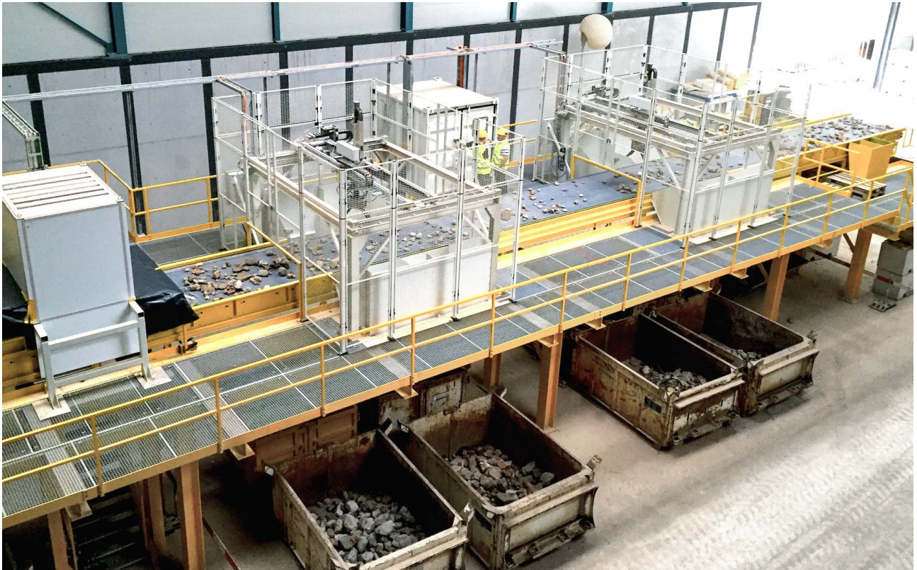
Sorting belt for fully automated robot sorting
