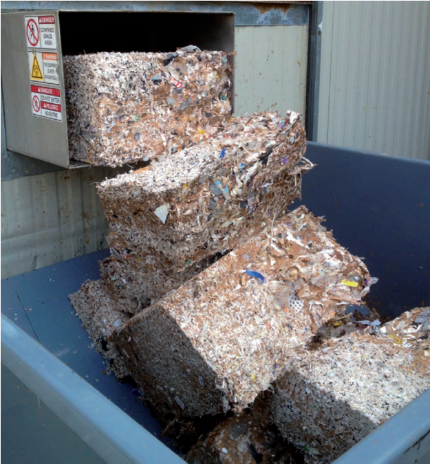
Dewatered pulp rejects
