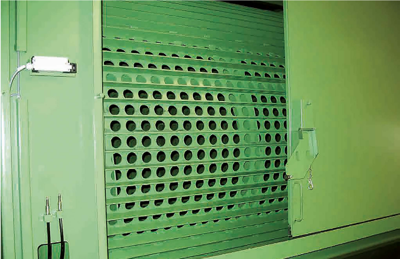
Screening drum with winding protection
