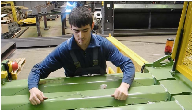
Manual binding with prefabricated quick-tie wires
