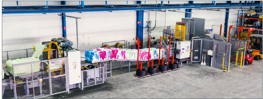
Fully-automated pressing and wrapping system
