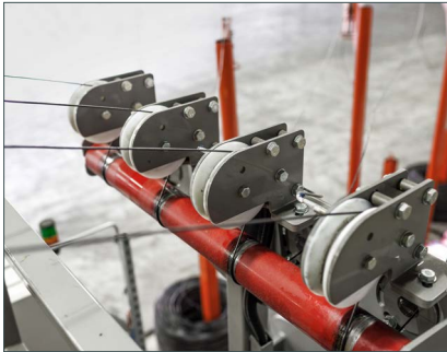
Monitoring of wire breakage and wire end to control the binding wires
