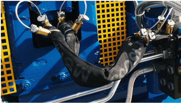
Hydraulic hose with safety trap and burst protection
