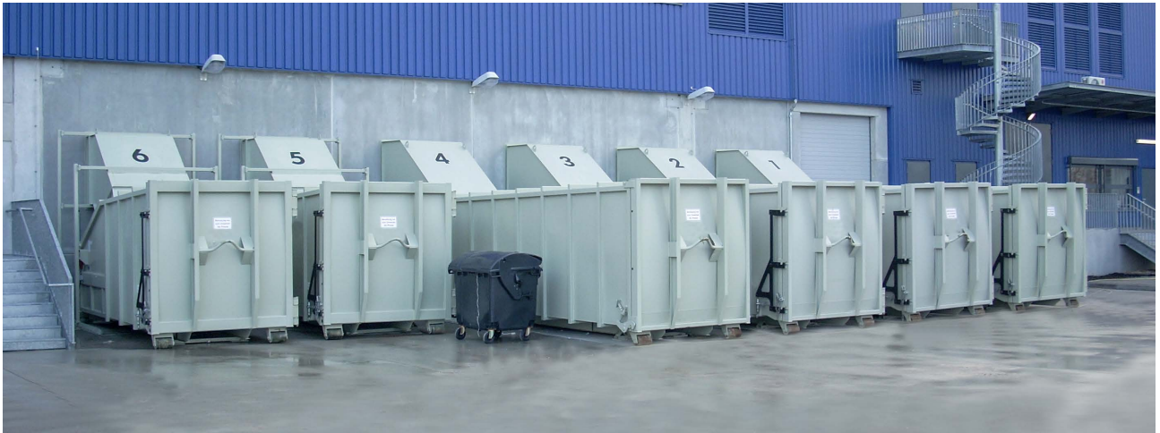
Transport containers at static compactor facility
