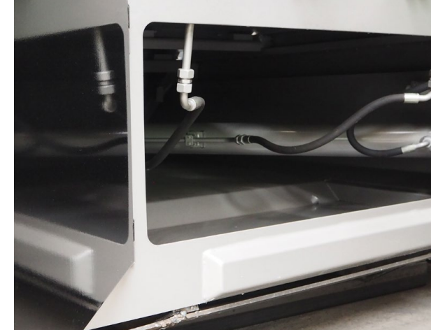
Self-cleaning tray in the press head
