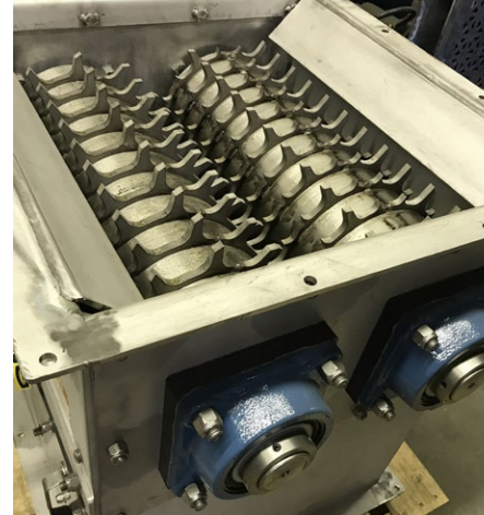
Robust 10mm stainless steel teeth
