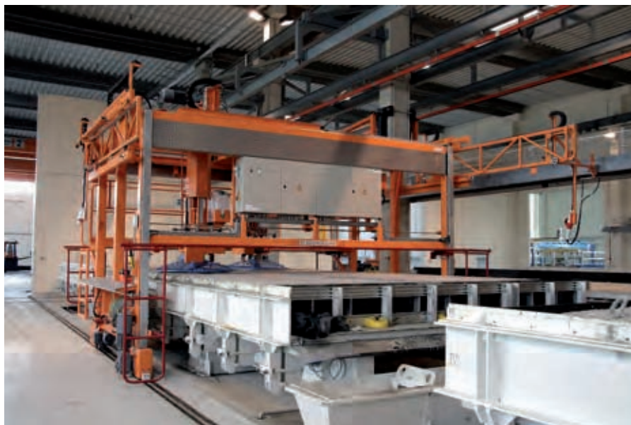
Radio controlled power trowel with 2 smoothing units
