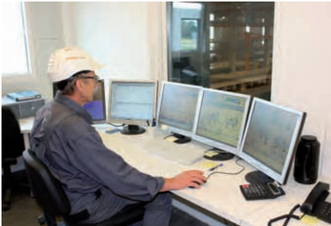
The Skakomat 600 controller organises all mixing processes
