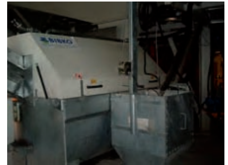
Recycling plant, type ComTec, with pump sump
