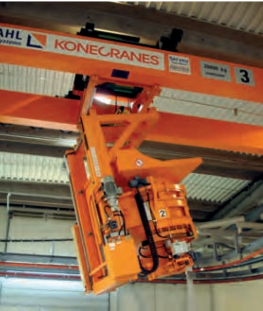
Concrete distributor being coupled to the crane
