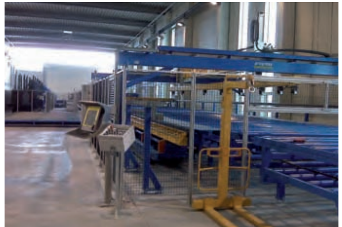
Meshes with dimensions of up to 6 m x 12 m can be produced on the mesh welding plant
