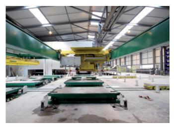
Vibratory compactor and concreting bay with concrete spreader
