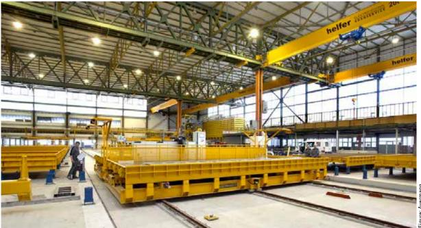
BWE-Bau produces a wide range of extensive precast elements, including solid walls and sophisticated sandwich façade panels as well as elaborate custom elements. The company primarily serves the residential segment, but the dimensions of the pallets used in the production process also allow for the manufacture of large-scale wall units for industrial premises.
