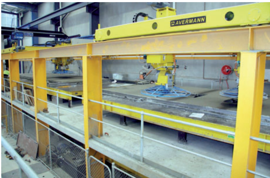
Smoothing bay with wing-type smoothing devices
