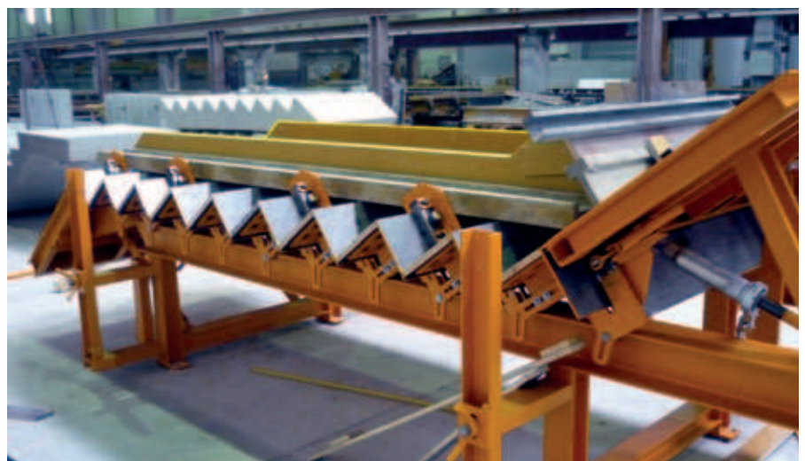
Fig. 2 Standard staircase production
