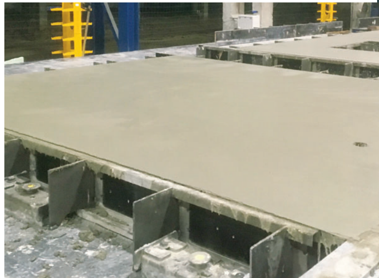
Smoothed concrete component
