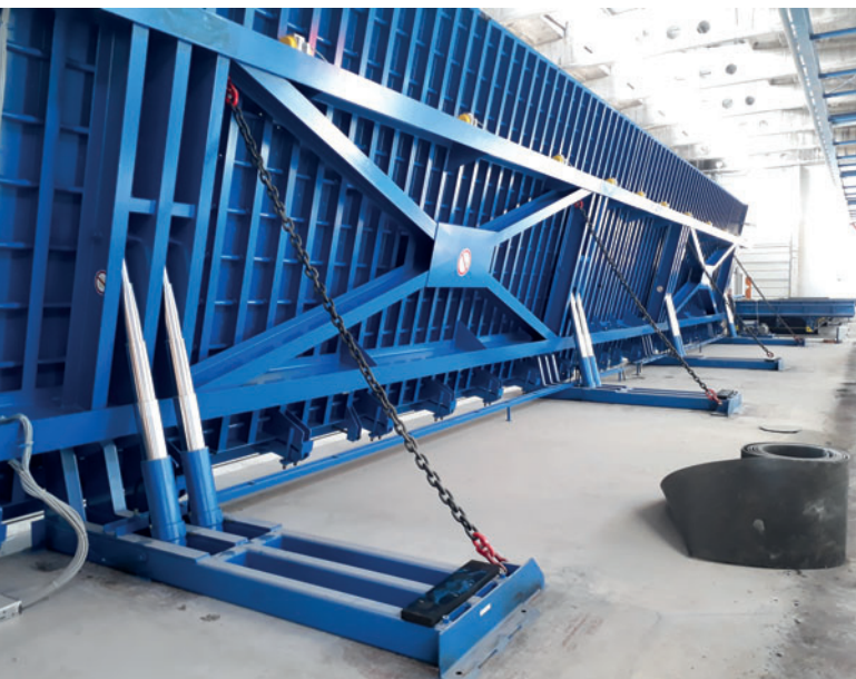
Tilting table line for producing walls
