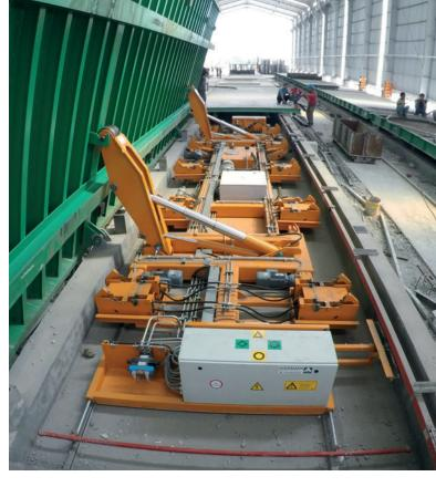
The titling-compacting machine's hydraulic device tilts the table on its pivot points up to an angle of 80° so that the hall crane can hoist finished wall panels undamaged from the formwork table.
