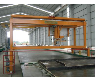
The tilting table system includes this power trowel, which gives the necessary high quality to the rear sides of these flat precast concrete elements
