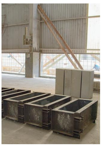
Residual concrete is utilised by PT Motive Mulia for a by-product - kerbstones (at the rear) - that separate pavements from the road carriageway in the capital, Jakarta. The company makes its own steel moulds (in the foreground) for this purpose.
