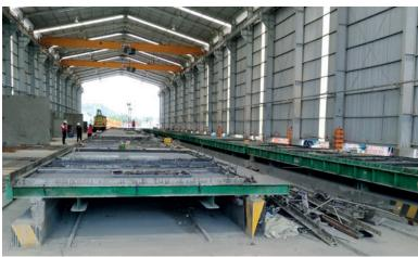
16 tilting tables are set up on two lines running parallel to each other in the production hall.
