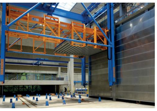
Storage and retrieval machine for hardening chamber feeding
