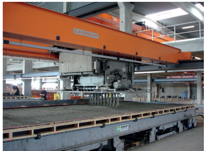
Fig. 5: Concreting station with concrete spreader and Avermann vibration compactor
