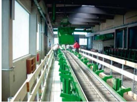
**Fig. 2** The new hydraulically powered base frame formwork in operation at the Glass factory.
