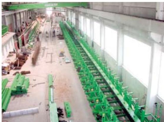
Fig. 1 Installation of the 72 m long base frame formwork by Avermann.
